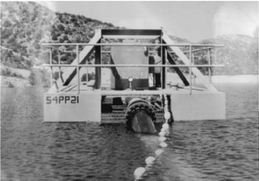
FIGURE 7 Unique design float-mounted pump (Hazleton Pumps, Inc.)
