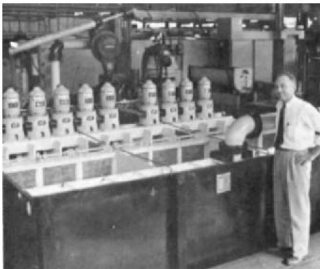
FIGURE 17 Model pit test setup with fixed screens and pumps and valves for variable flow, to scale (Flowserve Corporation)
