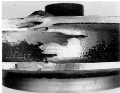
FIGURE 12 Erosion at the exit vane tips of a duplex, stainless steel CD4MCu impeller in a bauxite service.
