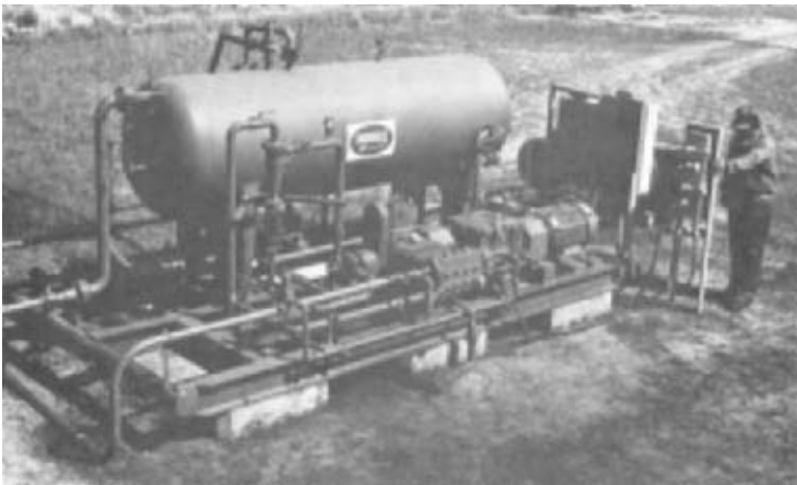
FIGURE 10 One-well unitized system (National Supply)
