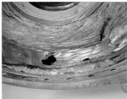
FIGURE 11 The severe erosion of a carbon steel casing in a 17% bauxite and sand service. Note the gouging due to the local turbulence of the slurry.
