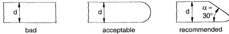
Fig.G.4.4 Recommendations for profilation of trailing edge of ribs and outlet of diffuser vanes
